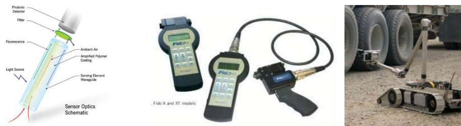
Figure 7: From left to right; the first image is an illustration of the sensing element within the Fido technology. The second picture is the handheld Fido XT sensor system that is available as COTS used in many applications. The third image is from the ICx technologies marketing brochure that demonstrates the capability to remotely deploy Fido-based sensor systems. [6]
