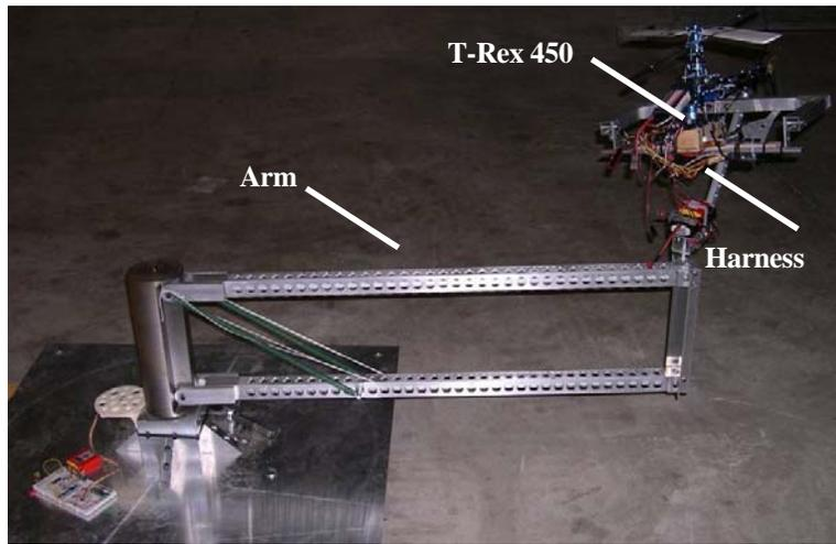
Figure 3: Ground-based Flight Test Stand with T-Rex 450
