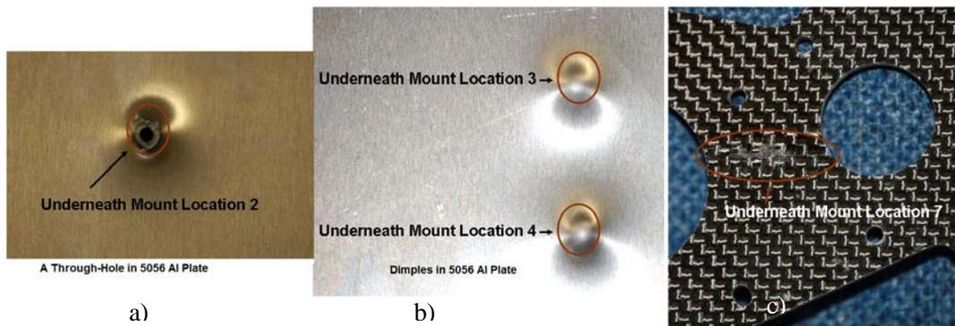
Figure 4: a) & b) Underneath M100 Test on Flat Al 5056 Plates c) on Composite Raptor 90 Side Plate
