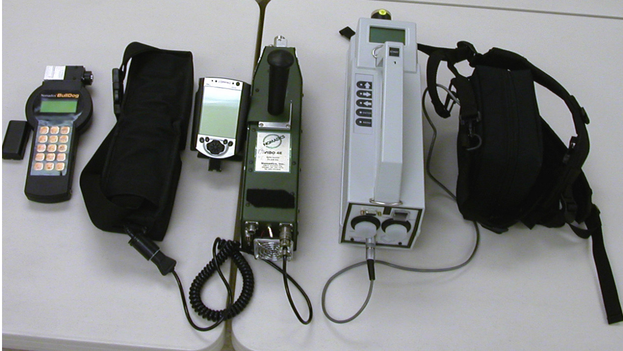
Figure 1. Comparison of trace chemical sensors and batteries. From left to right, the Fido X sensor (1.5 pounds), Fido 4EG sensor (previous Fido prototype, approximately 10 pounds), and commercial off-the-shelf ion mobility spectrometer (almost 20 pounds).
