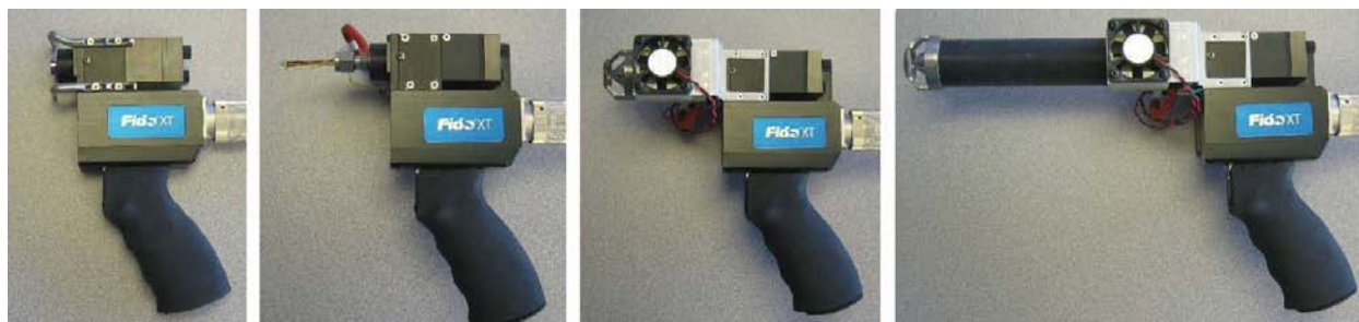
Figure 9: Evolution of the Fido XT Preconcentrator (Left to Right: Standard Fido XT, Fido XT CG5, Coiled GC Precon, Linear GC Precon)
