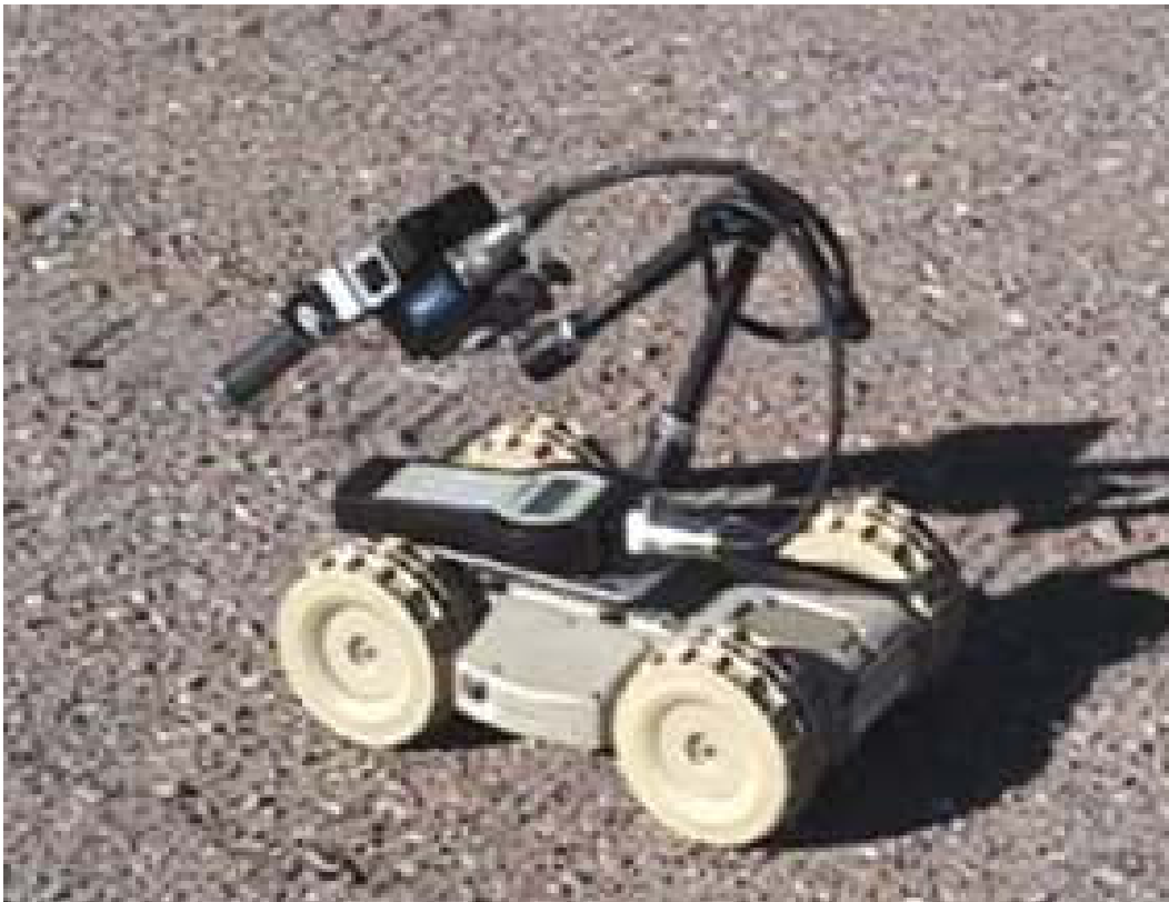
Figure 10: Fido XT GC Precon on the Dragon Runner at YPG Countermine Test Facility
