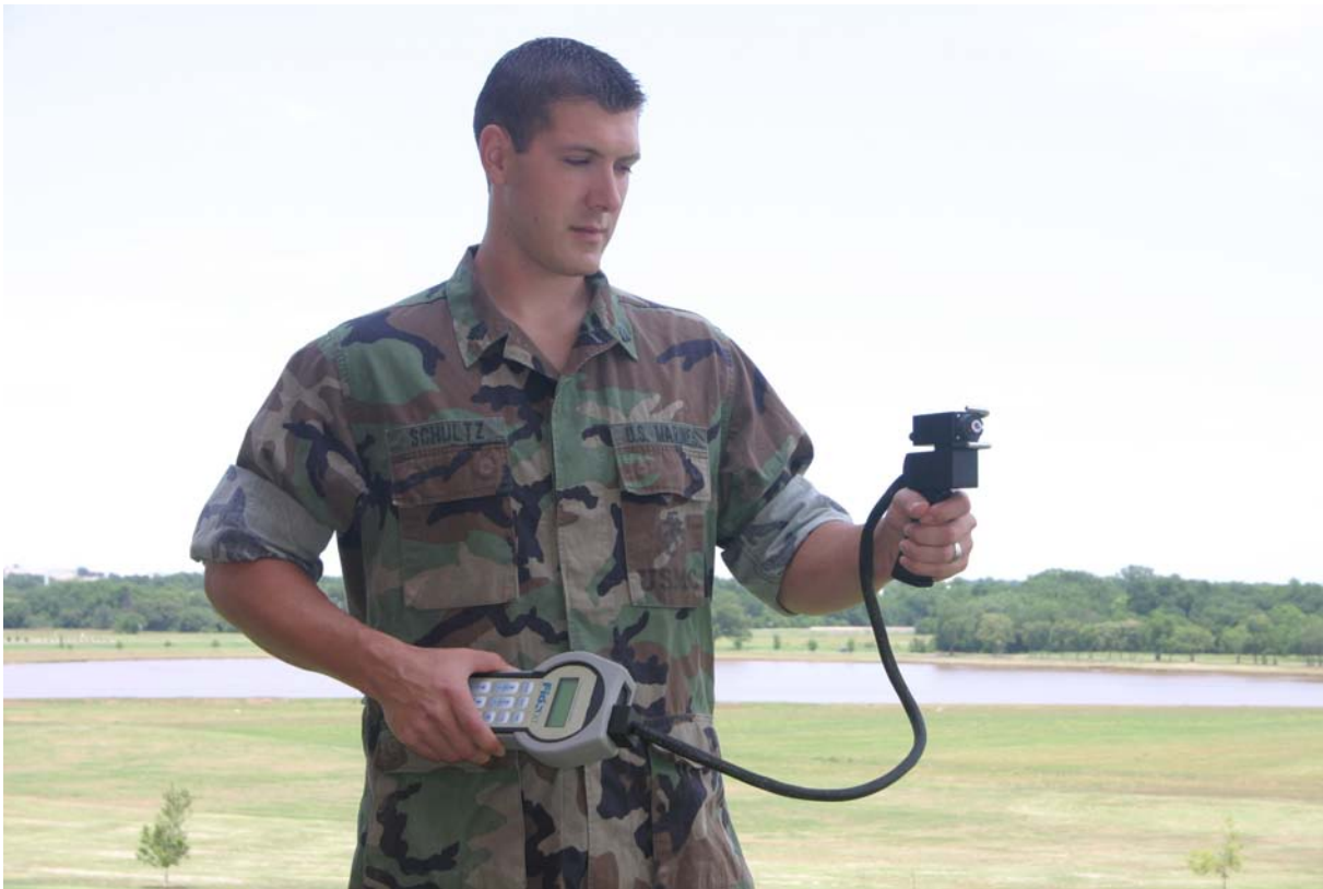
Figure 2. Fido XT operated in hand-held mode.
