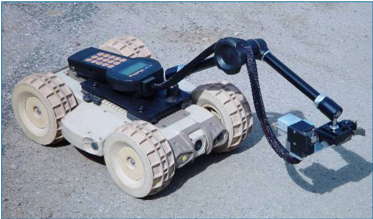
Figure 3. Fido XT deployed on the USMC Dragon Runner.
