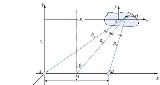
Fig. 1 Geometry of InISAR three-antenna imaging system
