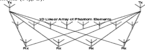
Fig. 2. An antenna array with physical 2 transmitting and 4 receiving elements and an equivalent array with 8 transmit/receive elements [2]
